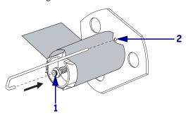
14. Rotate the spindle counterclockwise several turns to wind the media liner over the hook and remove any slack.
